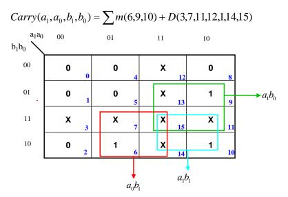
$$Carry(a_1, a_0, b_1, b_0) = a_0b_1 + a_1b_1 + a_1b_0$$
